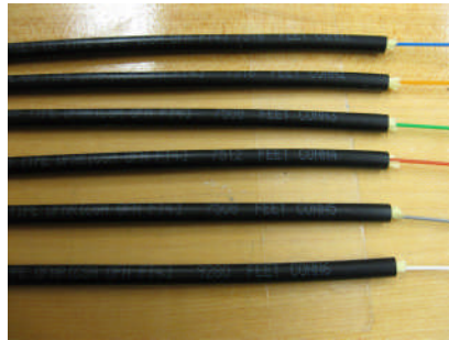
Cable identification and colored fiber.
